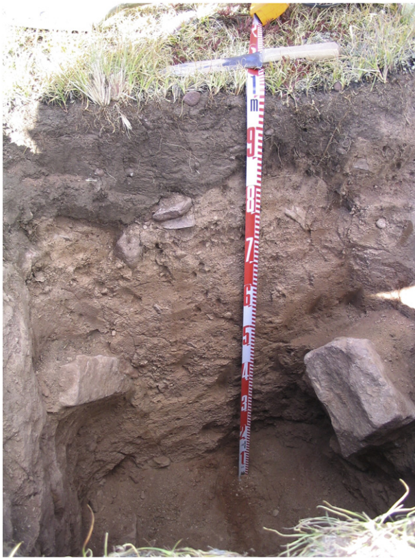
Fig. 2. Photograph of a representative soil profile in the alpine zone of the Uinta Mountains. A cap of stone-poor, silty material is clearly visible overlying a coarser subsoil. This surficial layer is interpreted as an alpine loess deposit.
