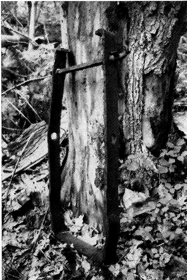
2-13. A unique binder assembly found among collapsed furnace debris at East Bennington. Note the key through the end of the spike (the other end of the spike is headed). Pairs of these binders were laid at right angles to each other in the corners of the stack to strengthen the walls.
