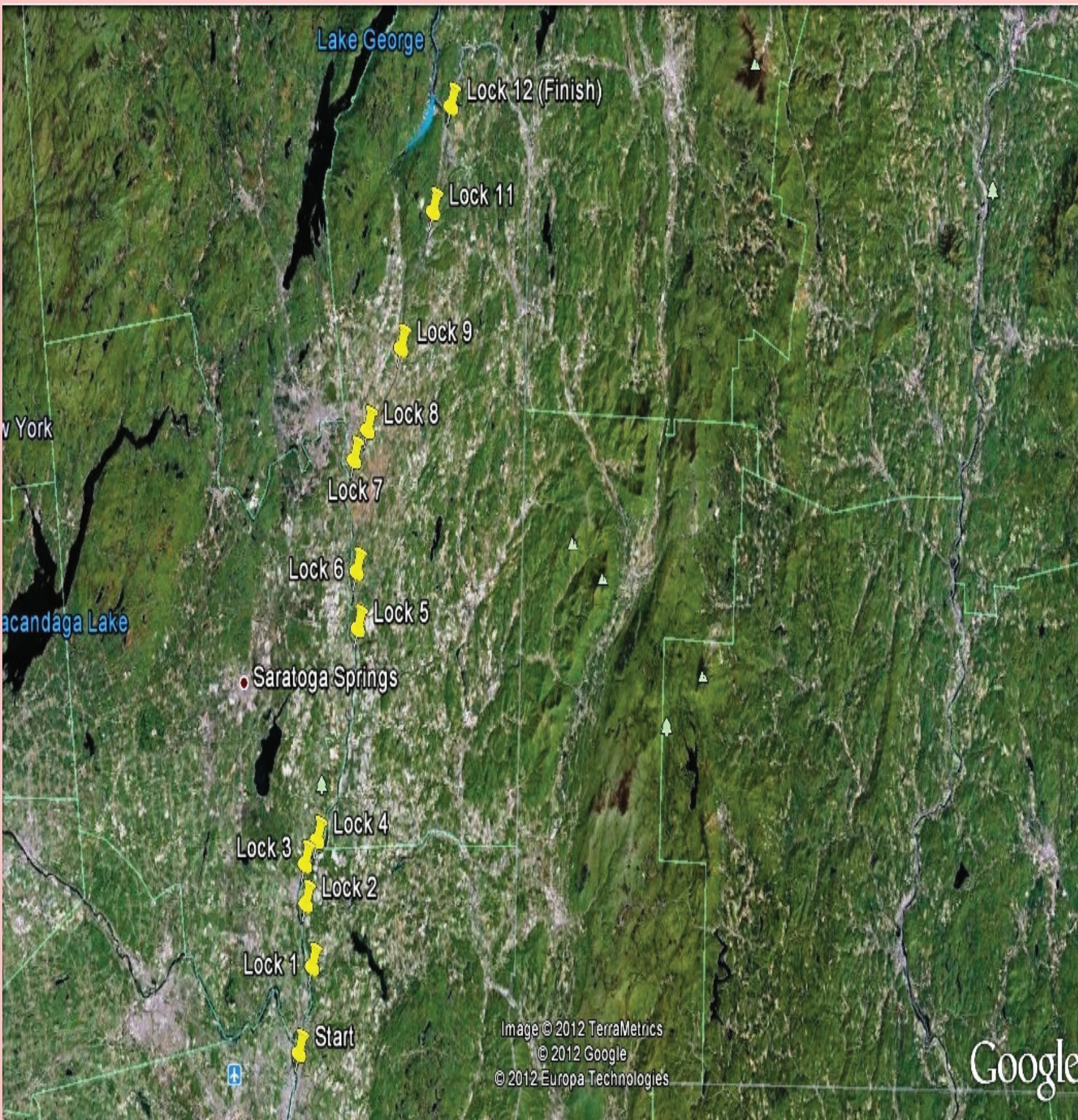
There are currently twelve locks on the Champlain Canal, as seen above. Nine were constructed between 1818-1823 and have been enlarged many times since, and three more were constructed in the early 1900s. Map modified from Google Earth.
