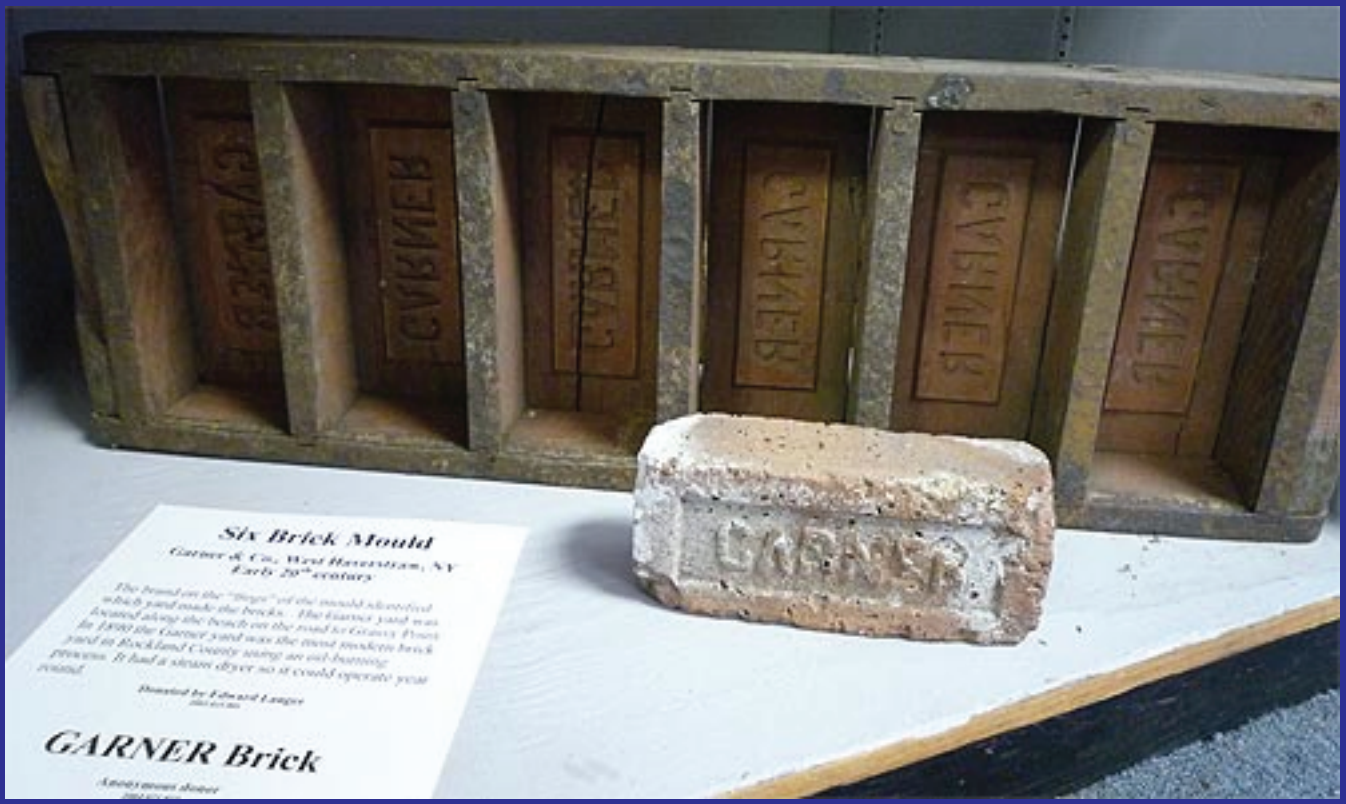
Figure 6. An example of an early wooden 6 brick mold. Laws were created early on to regulate the size of bricks to 9 inches in length, 4 ¼ inches in depth, and 2 ½ inches in height. Such regulation made it easier for bricklayers to complete projects accurately.
