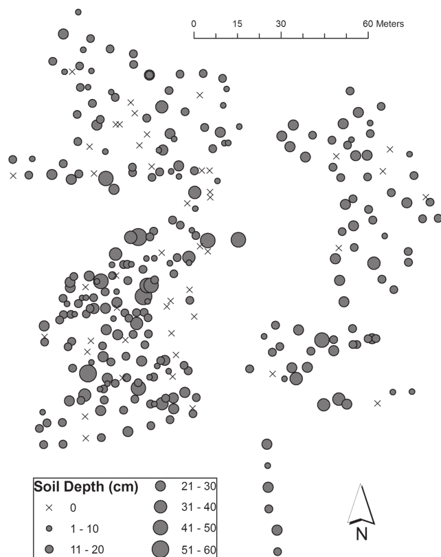
Fig. 4. Distribution of measured soil thickness in the study area based on 303 individual probings with a graduated steel rod. Deeper soils tend to found in isolated pockets, while shallower soils cluster in more contiguous areas. The central swath was intentionally skipped to avoid measuring soils potentially impacted by foot traffic along a major hiking trail.
